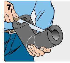
Calculate the tube's external diameter and 2 trace two parallel lines this far apart in the middle. Draw a line between the two to mark the centre line. Ø Then make two marks (C and D) either side of the centre line one centimeter from it, and draw two lines running
