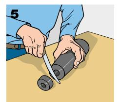
Shorten the other end, too, so that the coupling can be inserted neatly into the space left between the two existing sections.
