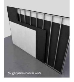
K-FLEX® glue to GK/GV and to the metallic surface. Put the GK/GV on the metallic panel. A 50mm overlap between two consecutive panels will give better results avoiding acoustic bridges. For thicker material (over 4kg/m<sup>2</sup> weight) use additionally a mechanical fixing with screws or pins every 50cm.
