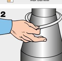
Measure the circumference of the widest pipe using a strip of K-FLEX<sup>®</sup> of the same thickness as the sheet.
