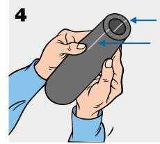
After positioning it on the pipe, glue the edges of the lengthwise cut with K-FLEX<sup>®</sup> glue and bond the edges of the sleeving to the other two sections of tubing.
