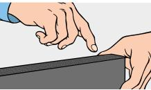
If the tube is not very long, or is not very thick, it can be rolled up and glued. This way, the tube can be quickly and easily applied to the pipe.
