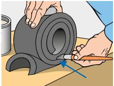
When attaching the two surfaces, press them together firmly with your fingers, starting at the far ends, then the centre and lastly along the intermediate points to avoid an irregular joint.
