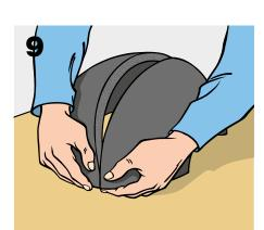
Wrap the K-FLEX® insulation around the pipe and press the edges tightly together.
