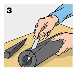
Cut the coupling along its length to install it on the pipe.
