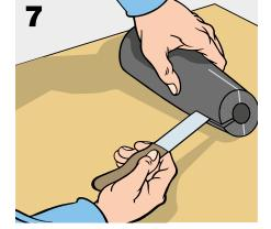
Glue the edges of the cut-outs together so that the diameter of the tubing reduces.
