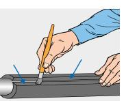
After spreading the glue, ensure that it has dried properly before attempting to stick the edges together. The best test is by touching the surface with your finger: if K-FLEX<sup>®</sup> glue no longer sticks to your finger forming threads, it is ready to be positioned.
