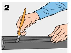
Cut the insert along its length and glue into place.
