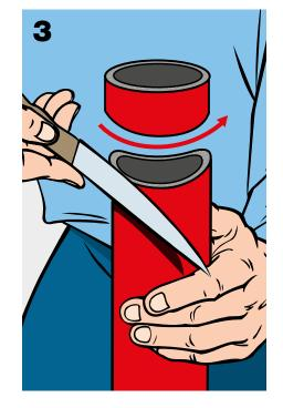
Cut the tube along its length and slide it onto the pipe so that the hole is positioned around the third pipe. Then stick the edges back together.
