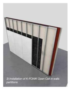
panel. For thicker material (over 30mm thick) use additionally a mechanical fixing with screws or pins every 50cm. Open Cell can be glued also on GK/ GV substrate Apply K-FLEX® glue to K-FONIK OPEN CELL and to the GK/ GV surface. Put the K-FONIK OPEN CELL on the panel. For thicker material (over 30mm thick) use additionally a mechanical fixing with screws or pins every 50cm.
